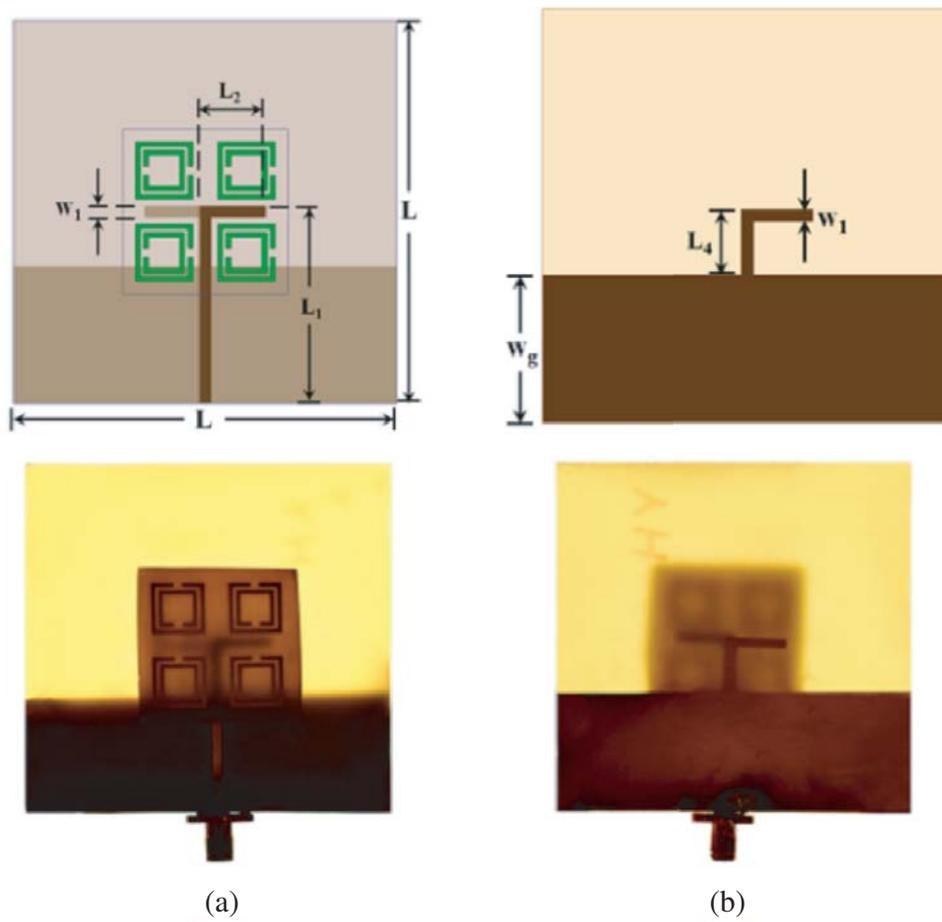
**Figure 3.** Schematic topology and fabricated prototype of the loaded antenna. (a) Front view. (b) Back view.
