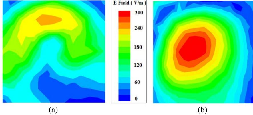
**Figure 7.** Simulated electric field distribution at the respective resonance frequency. (a) Reference antenna. (b) Metamaterial loaded antenna.
