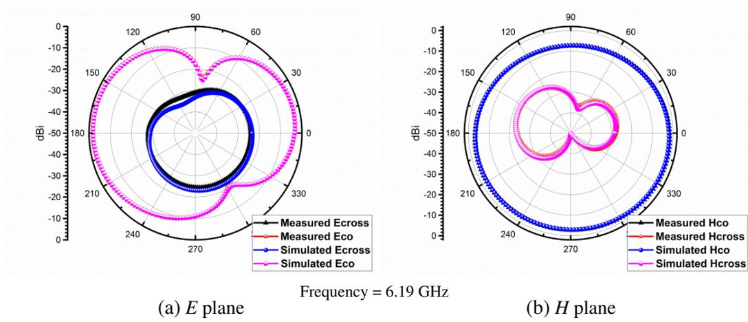
**Figure 6.** Simulated radiation pattern of the proposed antenna for (a) Eco (Elevation plane,  $XZ$  plane,  $\theta = 90^\circ$ ) plane and Ecross (Azimuthal plane,  $XY$  plane,  $\theta = 0^\circ$ ) plane, (b) Hco (Azimuthal plane,  $XY$  plane,  $\varphi = 0^\circ$ ) plane and Hcross (Elevation plane,  $XY$  plane,  $\varphi = 90^\circ$ ) plane.
