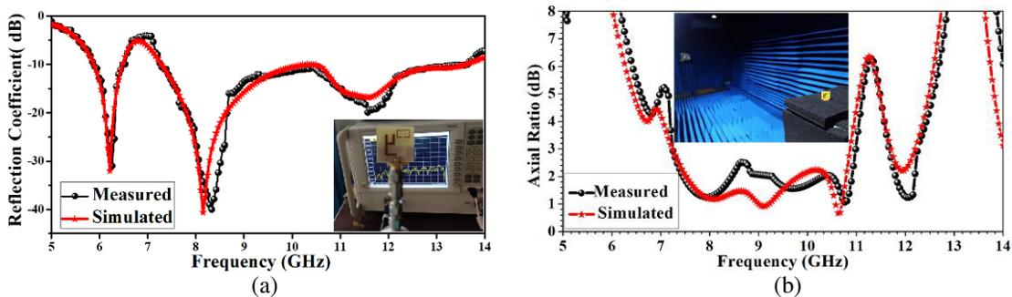
**Figure 4.** Comparison of measured and simulated (a) reflection coefficient curves and (b) ARBW curves.
