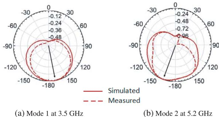
**Figure 7.** Simulated and Measured 2D  $H$  plane Normalized radiation pattern in dB to illustrate pattern reconfiguration in various switching modes.
