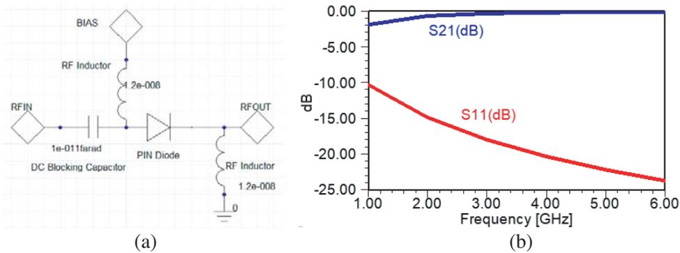
**Figure 4.** (a) PIN diode biasing circuit. (b)  $S_{11}$  and  $S_{21}$  Graph of PIN diode.
