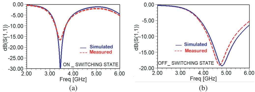
**Figure 5.** Simulated and measured value of  $S_{11}$  in dB. (a) ON state. (b) OFF state.
