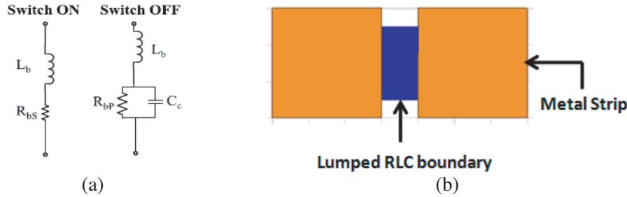
**Figure 3.** (a) Equivalent circuit of PIN diode. (b) PIN diode model in HFSS.
