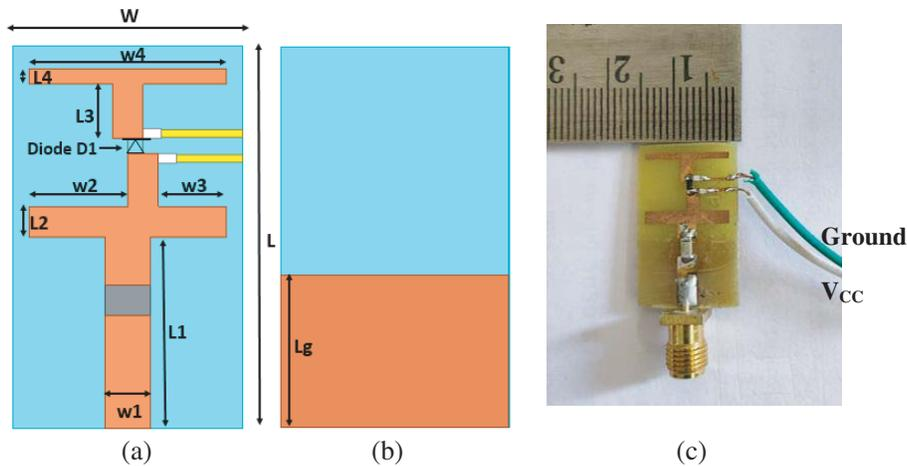
**Figure 1.** Proposed antenna. (a) Top view (Grey-capacitor, White-inductor, Yellow-biasing strips). (b) Bottom view. (c) Fabricated antenna.
