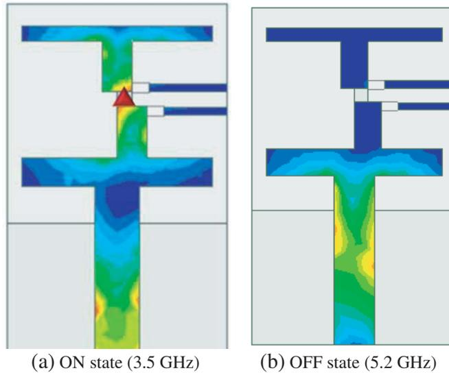
**Figure 6.** Simulated electric field distributions for ON/OFF switching modes.
