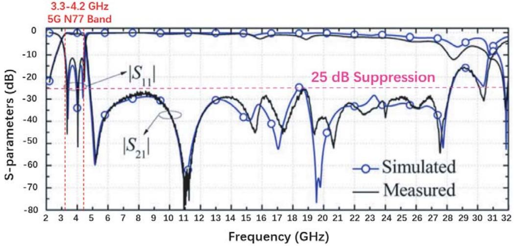
**Figure 5.** Simulated and measured results of proposed BPF.
