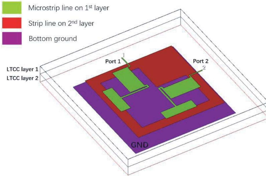
**Figure 1.** 3D structure of the proposed dual-mode BPF.
