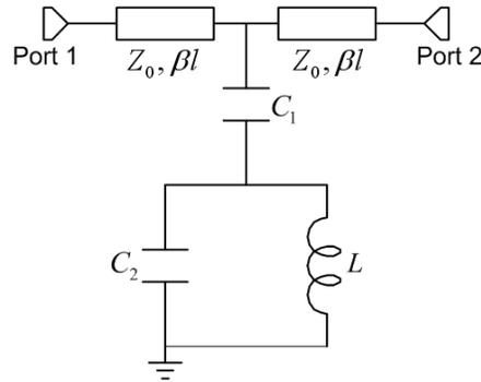
**Figure 2.** Equivalent circuit of suspended microstrip over an EBG unit.
