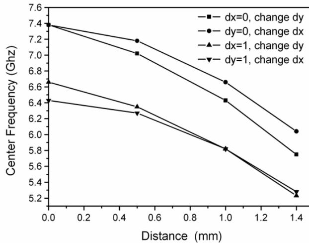
**Figure 4.** Center frequency changes with the position of via.
