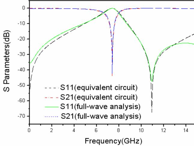
**Figure 3.** Comparison of equivalent circuit with full-wave analysis.
