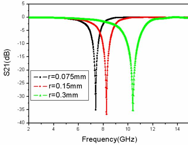
**Figure 5.** Center frequency changes with the radius of via.
