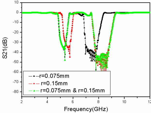
**Figure 8.** Comparison of cascaded structures with different radius of via.
