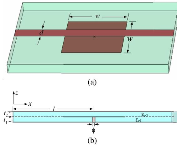
**Figure 1.** Geometry of suspended microstrip over an EBG unit. (a) 3D view. (b) side view.
