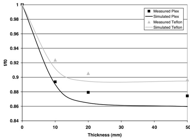
**Figure 5.** Resonant frequency of the patch sensor normalized to the resonant frequency of the unloaded patch, versus the thickness of the material used as a superstrate layer, when the latter has a relative permittivity  $\varepsilon_m = 2.1$  (Teflon) or  $\varepsilon_m = 2.6$  (Plexiglass). Simulation results obtained with CST Microwave Studio (continuous lines) are compared with experimental results (markers).
