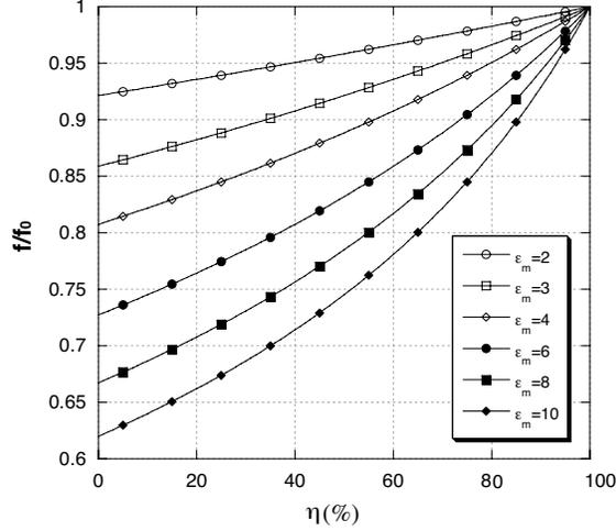
**Figure 4.** Resonant frequency of the patch sensor normalized to the resonant frequency of the unloaded patch, versus the porosity degree of the material under test and for different values of the relative permittivity of the intrinsic material (porosity free). The curves have been obtained by implementing Eq. (11).
