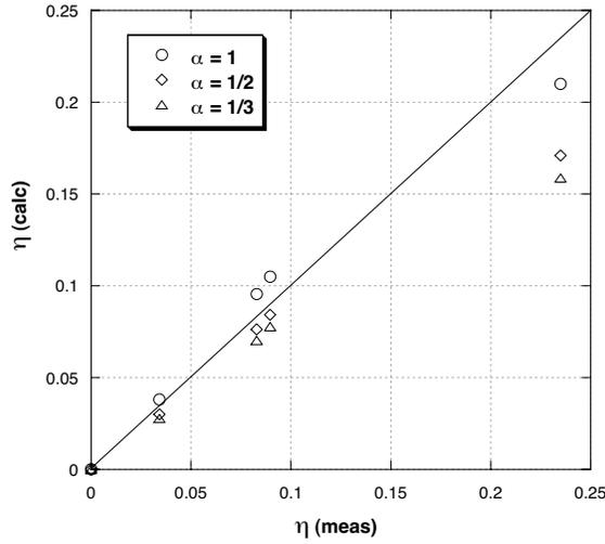
**Figure 3.** Porosity values,  $\eta$ , calculated with  $\alpha = 1/3, 1/2, 1$ , as a function of porosity values derived through the measurements of the sample mass and volume (see  $\eta\%$  in Table 1 and linear regression parameters in Table 3).
