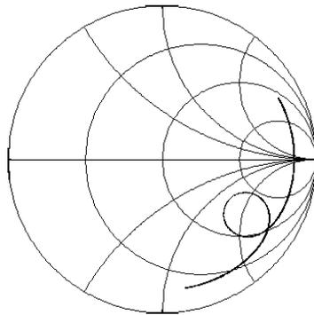
**Figure 5.** Measurement  $Z_i$  of the dielectric resonator in Smith Chart.
