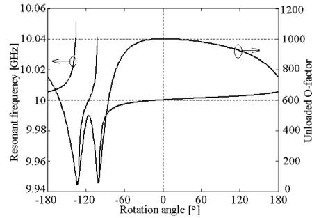
**Figure 4.** Resonant frequency and unloaded Q-factor versus rotation angle of simulation data.
