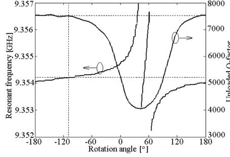
**Figure 10.** Resonant frequency and unloaded Q-factor versus rotation angle of the cylindrical cavity.
