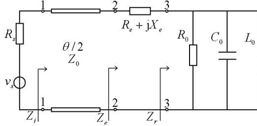
**Figure 1.** General equivalent circuit of microwave resonator including the feed line.
