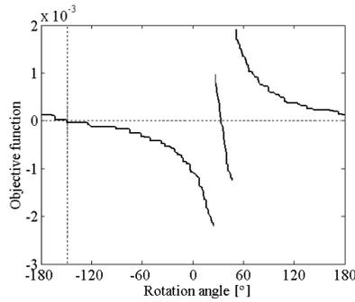
**Figure 6.** Objective function versus rotation angle of the dielectric resonator.
