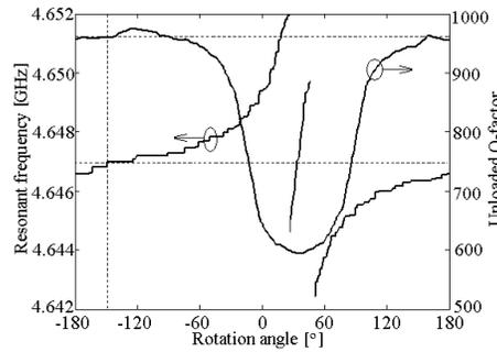
**Figure 7.** Resonant frequency and unloaded Q-factor versus rotation angle of the dielectric resonator.
