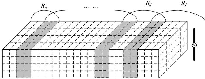
**Figure 3.** Multi-region model for antenna and dielectric box.
