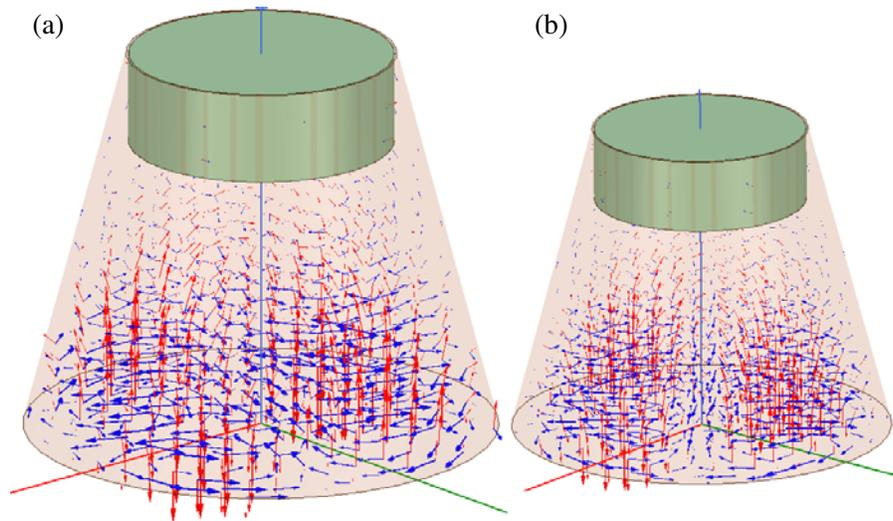
**Figure 3.** TM212 electromagnetic configuration simulated from the NASA cavity design (a) at 1974 MHz and (b) at 2450 MHz. Blue arrows represent magnetic field, and red arrows represent electric field.
