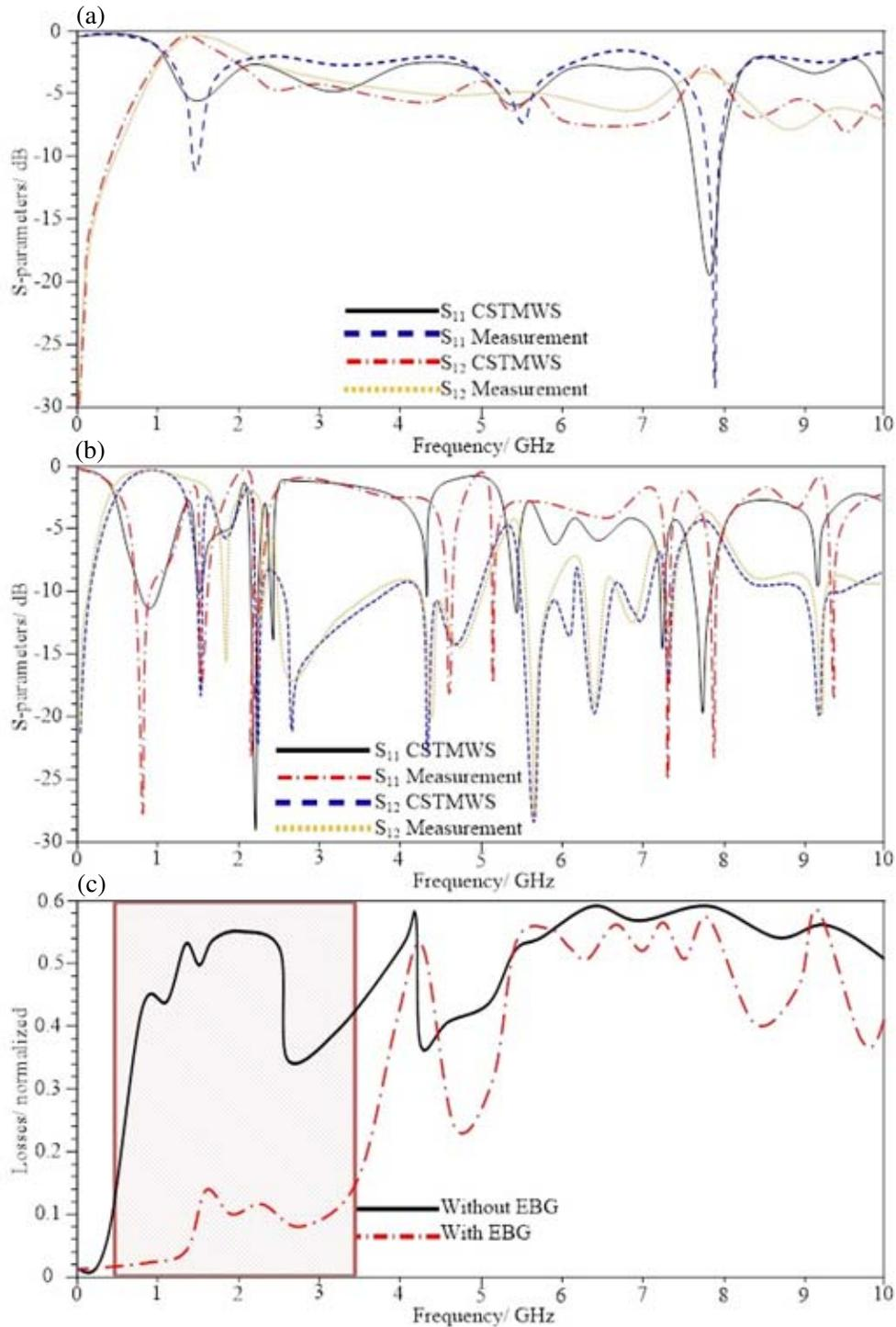
**Figure 3.** Evaluated losses based T-junction transmission; (a)  $S$ -parameters of the T-junction transmission without EBG structure, (b)  $S$ -parameters of the T-junction transmission with EBG structure, and (c) computed losses from the two proposed scenarios.
