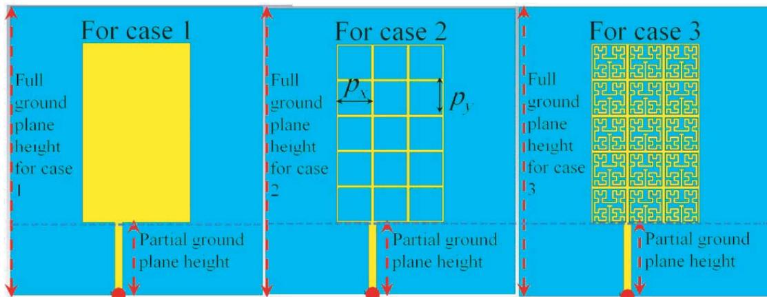
Figure 7. Numerical models of the proposed patches.
