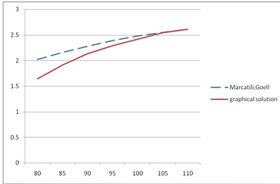
Figure 4. Normalized propagation constant ( $k_z/k_0$ ) versus frequency (GHz).
