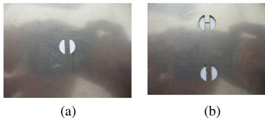
**Figure 8.** Photographs of apertures fabricated on a stainless steel plate: (a) Single aperture. (b) Dual apertures ( $Y_d = 29$  mm).
