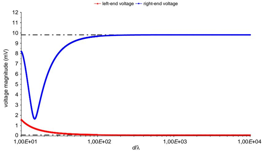
**Figure 4.** Plot of the left-end load voltage  $|V_0|$  and the right-end voltage  $|V_L|$  as functions of  $d/\lambda$  for the excitation field of (11)–(13) with  $x_0 = d$ ,  $z_0 = d + s/2$  and  $A$  given by (16). The parameters of the transmission line are  $b/\lambda = 0.03$ ,  $p/\lambda = 0.3$  and  $s/\lambda = 15$ . The line is terminated in matched loads ( $Z_0 = Z_L = Z_c$ ). The solid straight lines represent the plane-wave response for  $\theta_0 = 3\pi/4$ .
