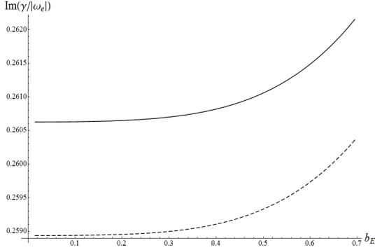
**Figure 3.** Growth rate of the SECTM-mode at the first frequency band  $1 < \omega/|\omega_e| < 2$  vs dimensionless amplitude of a pumping electric field  $b_E$ ;  $\omega_0 = |\omega_e|/2$ ;  $k_1\rho_e = 1$ . Solid and dashed curves relate to  $Z = \Omega_e^2\omega_e^{-2} = 50$  and  $100$ , correspondingly.
