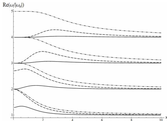
**Figure 1.** Eigen frequencies of the SECTM-modes vs normalized wave number  $x = k_1\rho_e$ ;  $b_E = 0.5$ ;  $\omega_0 = |\omega_e|/2$ . Solid, dashed, dot dashed curves relate to  $Z = \Omega_e^2\omega_e^{-2} = 1.5, 10$  and  $100$ , correspondingly.
