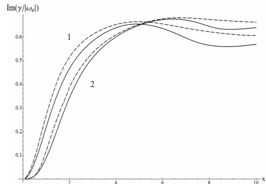
**Figure 2.** Growth rate of the SECTM-modes vs product  $k_1\rho_e$ ;  $b_E = 0.5$ ;  $\omega_0 = |\omega_e|/2$ . Solid and dashed curves relate to  $Z = \Omega_e^2\omega_e^{-2} = 1.5$  and  $10$ , correspondingly. Numerals 1 and 2 denote the series number of cyclotron harmonic  $s = 1, 3$ , correspondingly.
