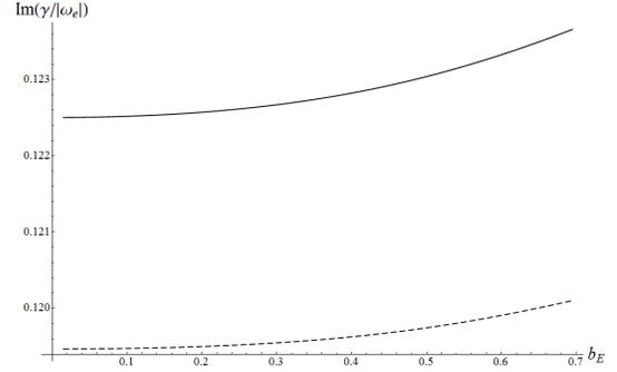
**Figure 4.** Growth rate of the SECTM-mode at the second frequency band  $2 < \omega/|\omega_e| < 3$  vs dimensionless amplitude of a pumping electric field  $b_E$ ;  $\omega_0 = |\omega_e|/2$ ;  $k_1\rho_e = 1$ . Solid and dashed curves relate to  $Z = \Omega_e^2\omega_e^{-2} = 50$  and  $100$ , correspondingly.
