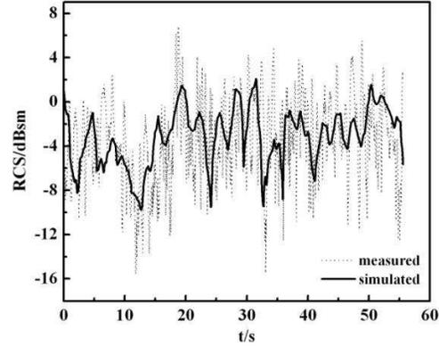
Figure 6. Comparison of measured and simulated RCS.
