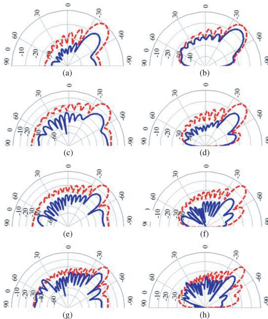
**Figure 5.** Comparison of simulated bistatic reflection between a metal sheet and a finite radome. (a) TE 7 GHz, (b) TM 7 GHz, (c) TE 9 GHz, (d) TM 9 GHz, (e) TE 12 GHz, (f) TM 12 GHz, (g) TE 15 GHz, (h) TM 15 GHz.
