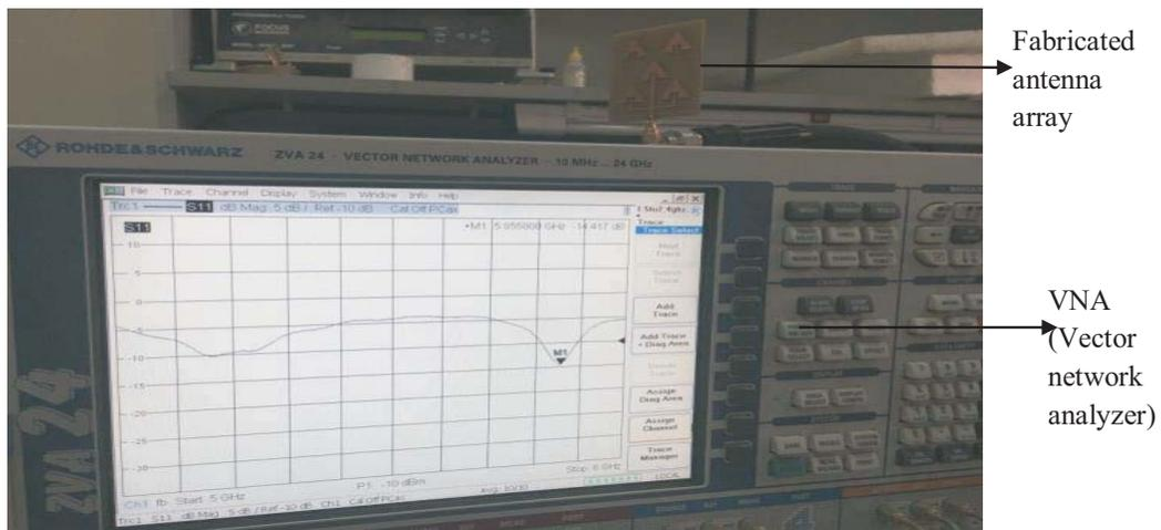
Figure 12. Experimental setup.
