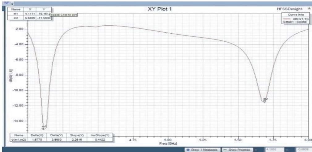
Figure 3. Simulated return loss of antenna element.
