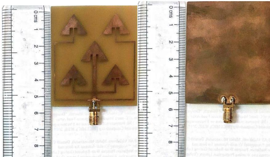
**Figure 8.** Prototype of realized antenna array.
