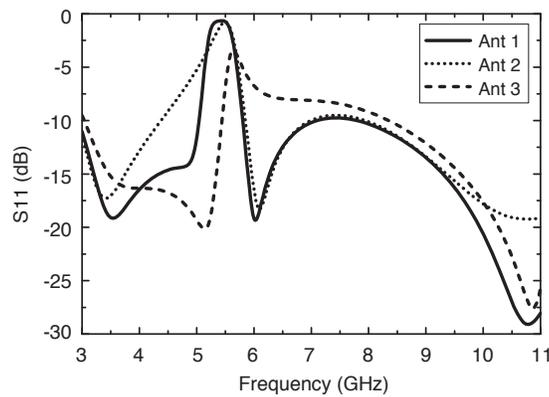
Figure 8. Reflection coefficient ( $S_{11}$ ) comparison of the band-notched antennas.
