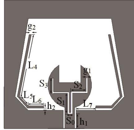
**Figure 6.** Schematic diagram of the band-notched UWB antenna.
