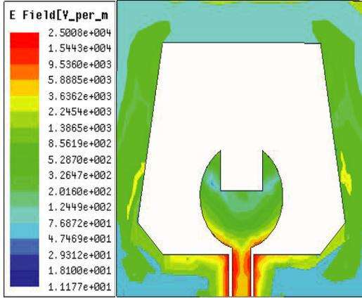
**Figure 5.** Surface current distribution of the UWB antenna.
