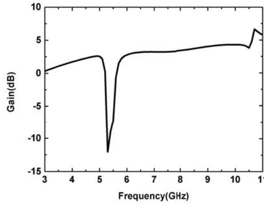
Figure 11. The simulated gain of the band-notched UWB antenna.
