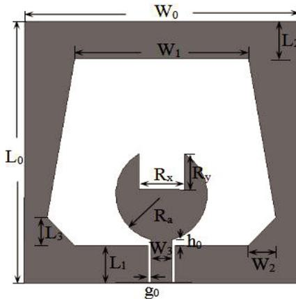
**Figure 1.** Schematic diagram of the UWB antenna.
