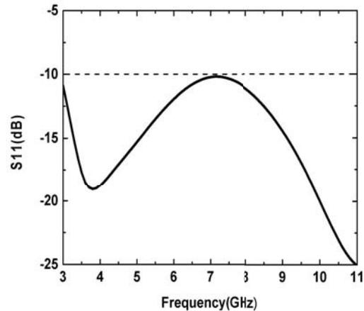
**Figure 2.** The simulated  $S_{11}$  of the UWB antenna.
