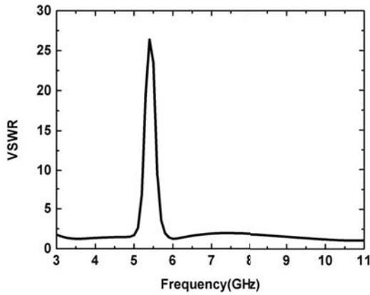
Figure 10. The simulated VSWR characteristic of the band-notched UWB antenna.
