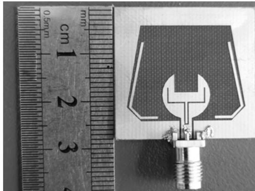
**Figure 13.** Fabricated sample of the proposed antenna.
