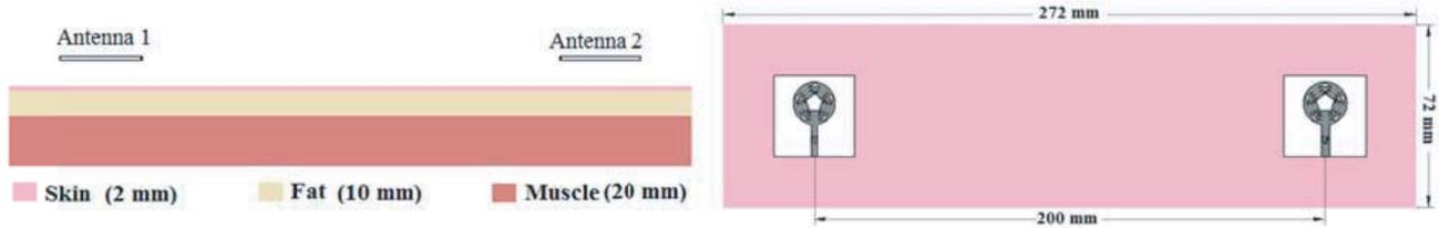
**Figure 4.** Three layered human tissue model for time domain analysis with identical antenna placed side by side at a distance of 5 mm from the skin (Front and Top view).
