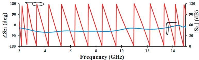
**Figure 6.** Magnitude and phase of  $S_{21}$  for antenna placed side by side on hand.
