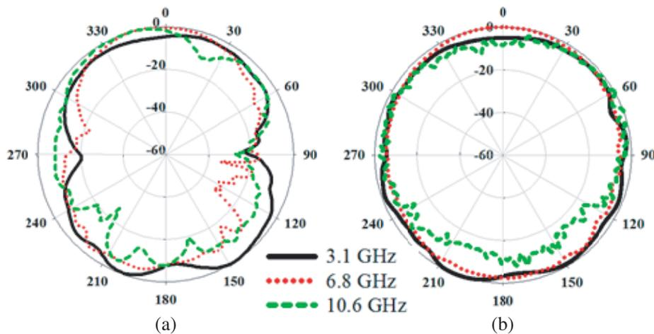
**Figure 3.** Measured radiation pattern of the proposed antenna (a)  $E$ -plane, (b)  $H$ -plane at 3.1, 6.8 and 10.6 GHz.
