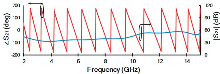
**Figure 5.** Magnitude and phase of  $S_{21}$  for antenna placed side by side in free space.
