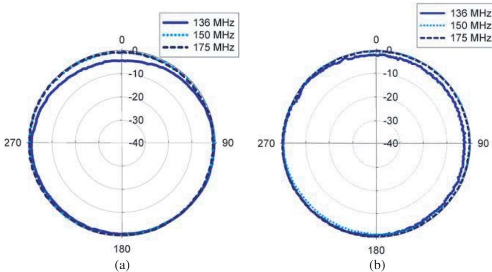
Figure 8. (a) Azimuth pattern with 4 ft ground plane. (b) Azimuth pattern without ground plane.
