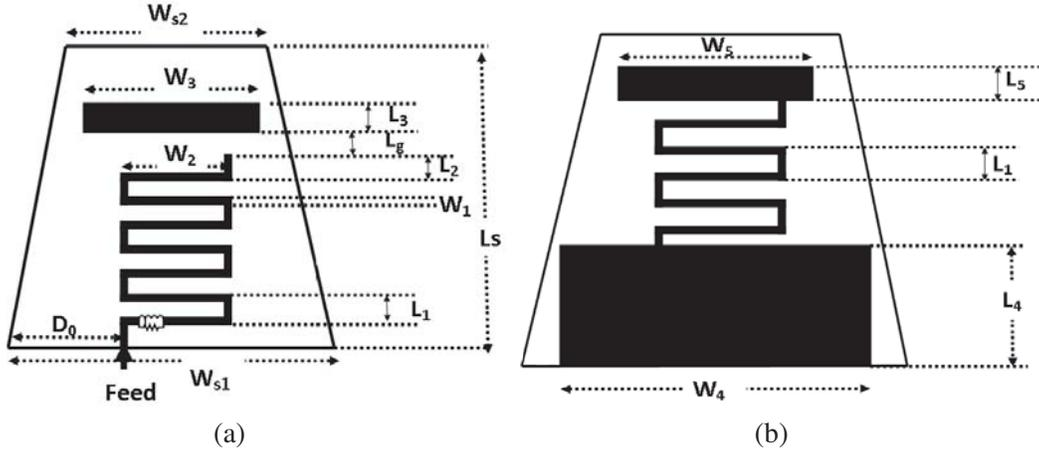
**Figure 3.** Structure of proposed antenna; (a) Radiating patch. (b) Ground patch.
