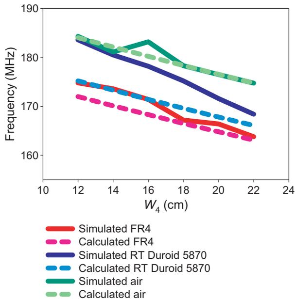
**Figure 15.** Comparison between theoretical and simulated result for various  $W_4$  values ( $h = 0.16$  cm;  $L_5 = 2$  cm;  $L_g = 1.5$  cm;  $L_3 = 2.5$  cm;  $L_4 = 9$  cm;  $W_3 = 14$  cm;  $W_5 = 15$  cm).
