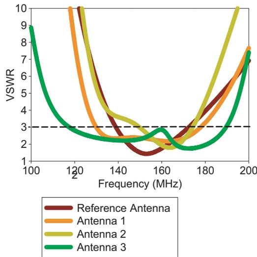
**Figure 2.** VSWR of antennas in the evolution process.
