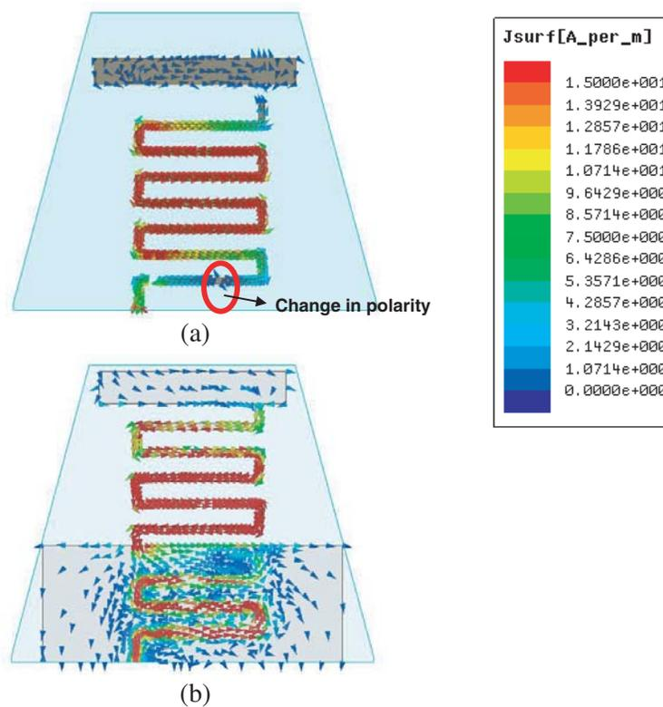
Figure 5. Simulated current distribution on (a) radiating patch, (b) ground patch.
