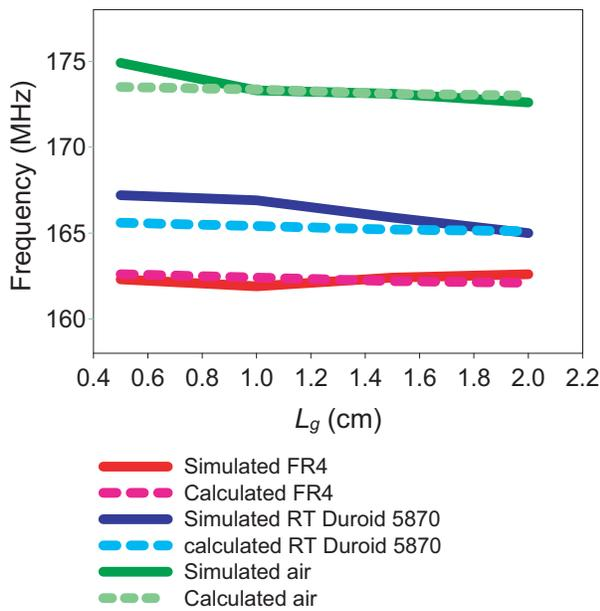
**Figure 11.** Comparison between theoretical and simulated result for various  $L_g$  values ( $h = 0.16$  cm;  $L_5 = 2$  cm;  $L_3 = 2.5$  cm;  $W_3 = 14$  cm;  $L_4 = 9$  cm;  $W_4 = 23.2$  cm;  $W_5 = 15$  cm).
