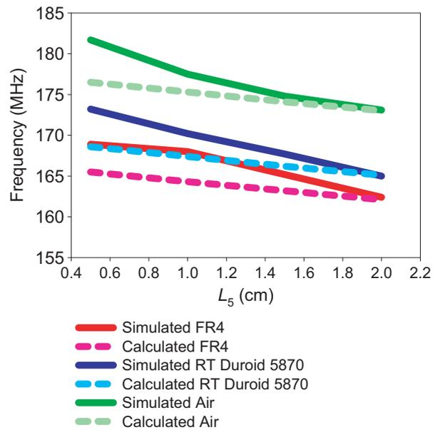
**Figure 16.** Comparison between theoretical and simulated result for various  $L_5$  values ( $h = 0.16$  cm;  $W_3 = 14$  cm;  $L_g = 1.5$  cm;  $L_3 = 2.5$  cm;  $L_4 = 9$  cm;  $W_4 = 23.2$  cm;  $W_5 = 15$  cm).
