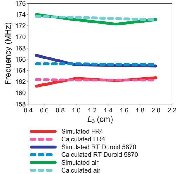
**Figure 12.** Comparison between theoretical and simulated result for various  $L_3$  values ( $h = 0.16$  cm;  $L_5 = 2$  cm;  $L_g = 1.5$  cm;  $W_3 = 14$  cm;  $L_4 = 9$  cm;  $W_4 = 23.2$  cm;  $W_5 = 15$  cm).
