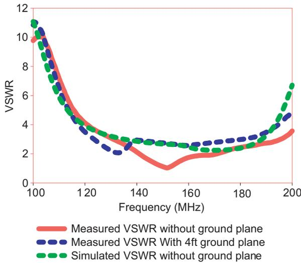
Figure 6. Measured VSWR with and without ground plane.
