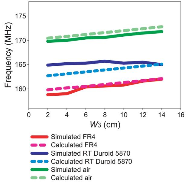
**Figure 14.** Comparison between theoretical and simulated result for various  $W_3$  values ( $h = 0.16$  cm;  $L_5 = 2$  cm;  $L_g = 1.5$  cm;  $L_3 = 2.5$  cm;  $L_4 = 9$  cm;  $W_4 = 23.2$  cm;  $W_5 = 15$  cm).
