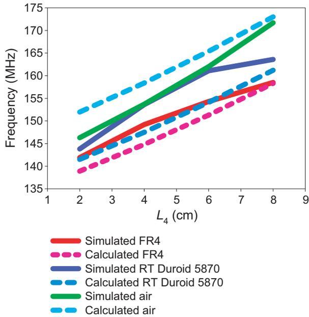
**Figure 13.** Comparison between theoretical and simulated result for various  $L_4$  values ( $h = 0.16$  cm;  $L_5 = 2$  cm;  $L_g = 1.5$  cm;  $W_3 = 14$  cm;  $L_3 = 2.5$  cm;  $W_4 = 23.2$  cm;  $W_5 = 15$  cm).
