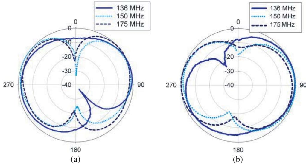
Figure 9. (a) Elevation pattern with 4 ft ground plane. (b) Elevation pattern without ground plane.
