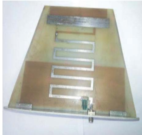
Figure 4. Photograph of fabricated antenna.
