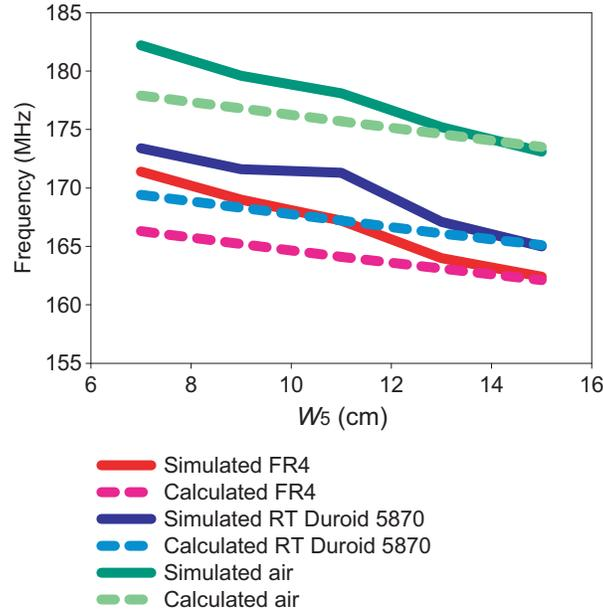
**Figure 17.** Comparison between theoretical and simulated result for various  $W_5$  values ( $h = 0.16$  cm;  $L_5 = 2$  cm;  $L_g = 1.5$  cm;  $L_3 = 2.5$  cm;  $L_4 = 9$  cm;  $W_4 = 23.2$  cm;  $W_3 = 14$  cm).
