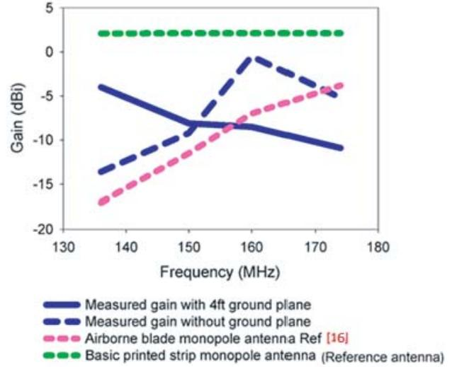
Figure 7. Measured gain.
