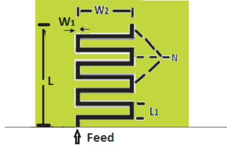
**Figure 10.** Structure of meander line antenna.
