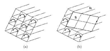
Figure 7. a) Family of parallel pipes representing even two-form. Orientation depicted as a curved arrow around axis of the pipe. b) Value of two form  $\mathbf{B}$  on bivector  $\mathbf{S}$ .
