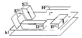
Figure 20. Configuration of relevant quantities for first eigenwave.
