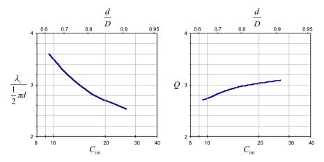
**Figure 8.** Normalised critical wavelength and Q for the TE-like mode in two-wire line.
