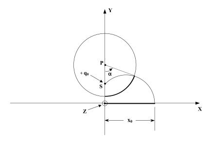
Figure D1. Geometry for determining resonator capacitance.
