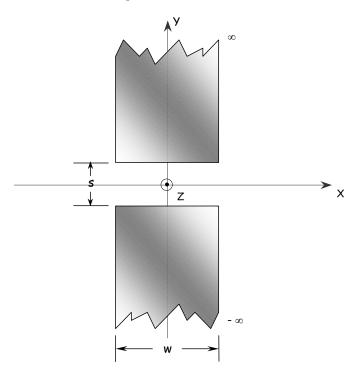
Figure 2. Slit in infinite slab.
