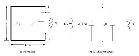
Figure 3. Equivalent resonator for the bifurcated parallel plate line.
