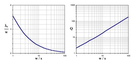
**Figure 6.** Normalised critical wavelength and Q in physical parallel plate line.
