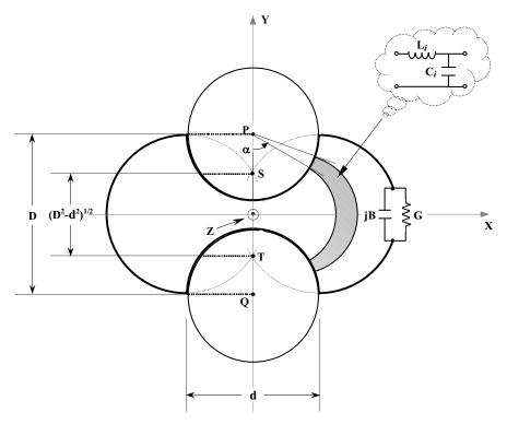
Figure 7. Resonator and its circuit representation.
