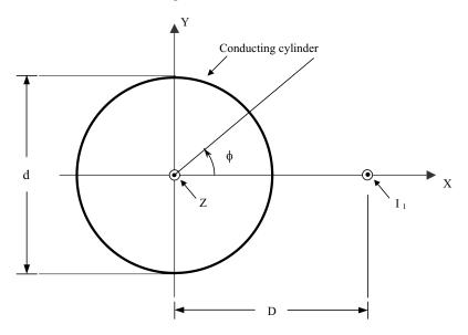
Figure 9. Wire parallel to cylinder-cross-sectional view.
