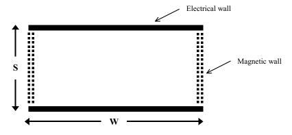
Figure 1. Prototype waveguide for perturbation.
