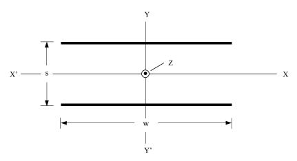
Figure 5. Physically realisable parallel plate line.
