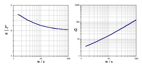
**Figure 4.** Normalised critical wavelength and Q in idealised parallel plate line.
