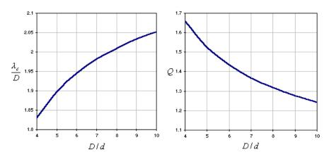
**Figure 10.** Normalised critical wavelength and Q in for TM-like mode in two-wire line.
