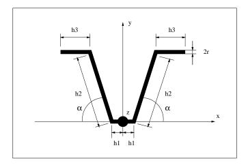
Figure 7. Geometry of the gull-shaped piecewise linear antenna.
