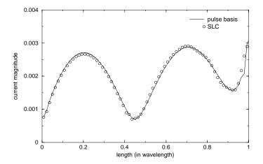
Figure 6. The normalized current magnitude: straight-wire antenna.
