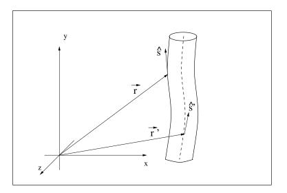
Figure 1. The thin-wire scatterer.
