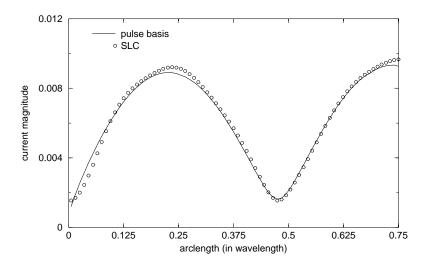
Figure 8. The normalized current magnitude versus arclength: gull-shaped antenna.
