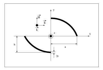
Figure 4. The thin-wire scatterer.
