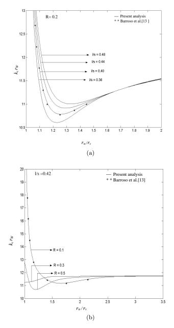
**Figure 3.** Variation of the eigenvalue of the typical waveguide mode  $TE_{6,2}$  with the ratio of the waveguide to ridge radii for configuration A, taking the slot width relative to the ridge periodicity (a) and the ridge depth relative to the outer ridge-edge radius (b) as the parameters.
