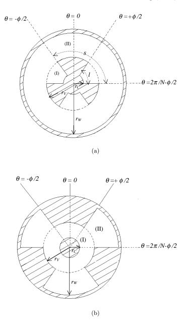
**Figure 1.** Cross section of a coaxial waveguide with ridged central conductor (configuration A) (a) and with vane-loaded outer conductor (configuration B) (b).
