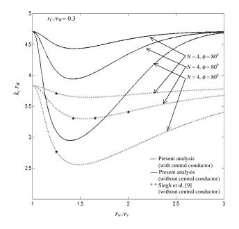
**Figure 4.** Variation of the eigenvalue of the typical waveguide mode  $TE_{0,1}$  with the ratio of the waveguide to ridge radii for configuration B, taking the vane dimensions as the parameters.
