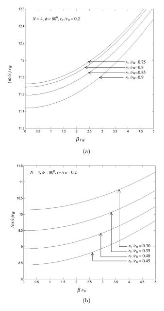
**Figure 2.**  $\omega$ - $\beta$  dispersion characteristics of a coaxial waveguide excited typically in TE<sub>6,2</sub> mode for configurations A (a) and B (b), taking the ridge/vane dimensions as the parameters.
