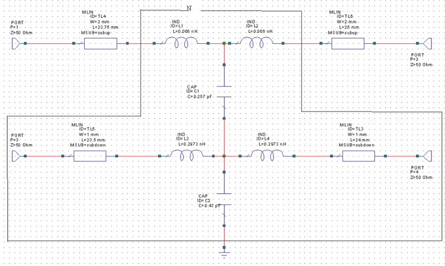
**Figure 6.** Equivalent two port network.
