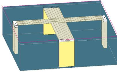
**Figure 1.** Two layer orthogonal microstrip transmission line.
