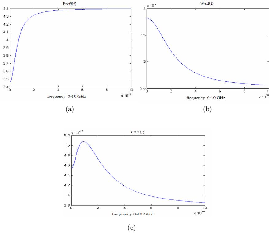
**Figure 5.** Plot (a)  $\epsilon_{reff}$  and (b)  $W_{eff}$  and (c)  $C_{12}$  variation in 1–10 GHz.
