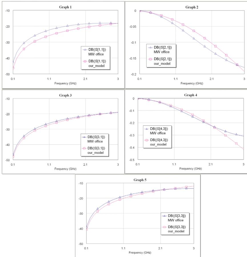
**Figure 7.** Comparing results of the equivalent circuit and physical structure.
