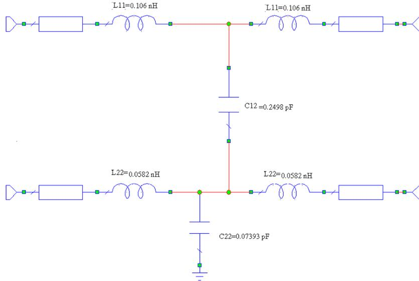
**Figure 2.** Equivalent circuit of two orthogonal microstrip lines in the cross talk region.
