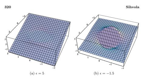
Figure 1. Potentials in the vicinity of the sphere with two different permittivities. Note the beginning of the development of a surface plasmon for the case of sphere with negative permittivity. As the permittivity decreases and passes the value -2, the internal field direction suddenly swaps and becomes opposite.
