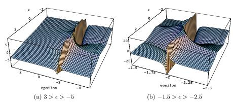
Figure 8. Potential through the center of a homogeneous sphere as a function of the permittivity. The sphere surface is crossed at  $z = \pm 1$ .
