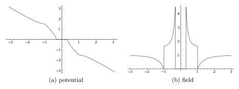
Figure 11. Potential and field for a hollow sphere with zeropermittivity shell.
