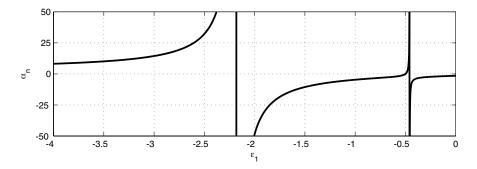
Figure 4. The polarizability of a plasmonic shell (as a function of its permittivity  $\epsilon_1$ ) which has a hollow core that occupies a volume of  $\beta = 0.03$ . Note the two resonances and the fact that the one closer to zero-permittivity is much narrower.
