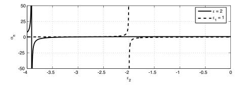
Figure 3. The polarizability of a plasmonic core (as a function of its permittivity  $\epsilon_2$ ) with a cover outside that has permittivity  $\epsilon_1 = 2$ . The core occupies a volume of  $\beta = 0.03$ . For comparison the polarizability curve of an uncovered sphere is shown with dashed line.
