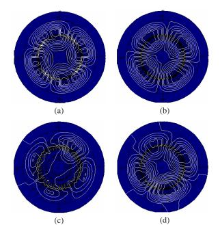
**Figure 6.** Flux distribution: (a) beginning of healthy motor starting, (b) steady-state operation of healthy motor, (c) beginning of faulty motor starting, (d) steady-state operation of faulty motor.
