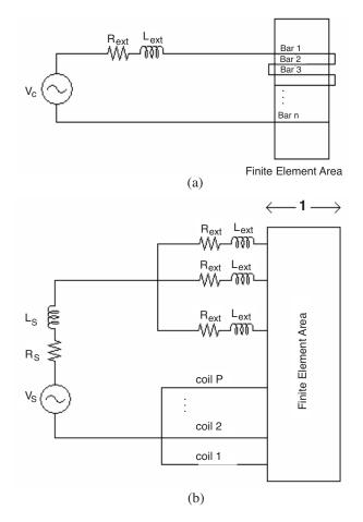
Figure 5. Forming coils: (a) series bars, (b) parallel bars.
