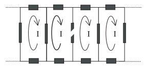
Figure 2. Distributed rotor cage in induction motor with one broken rotor bar.
