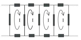
Figure 1. Distributed rotor cage in healthy induction motor.
