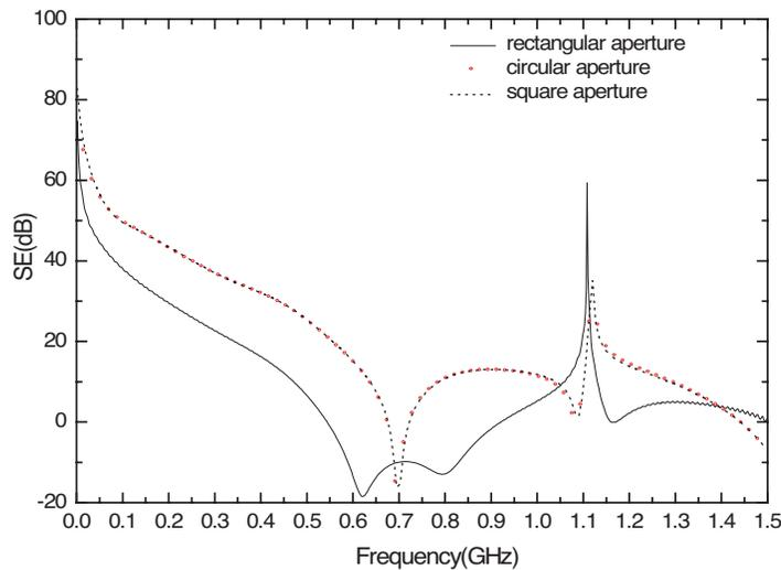
**Figure 15.** SE of the apertures with different shapes.
