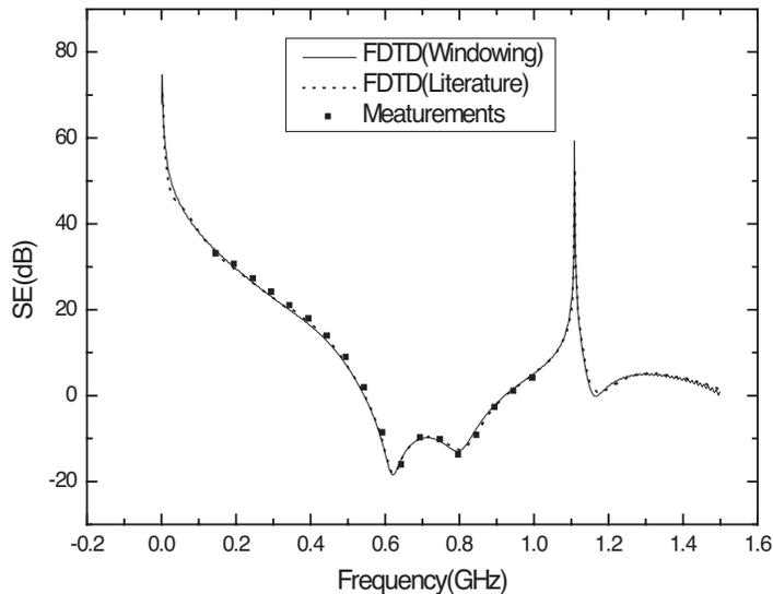
**Figure 10.** SE curve using Windowing technique.
