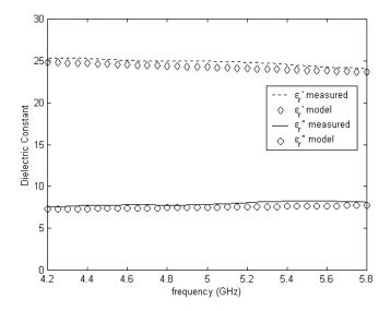
Figure 9. Measured dielectric constant of the leaf.
