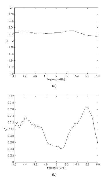
**Figure 8.** Measured dielectric constant (a) real part, and (b) imaginary part, of 0.5-mm thick Teflon.
