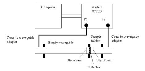
Figure 7. Measurement system setup.
