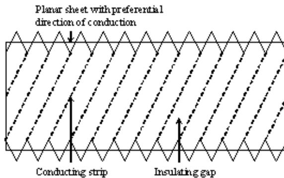
Figure 3. Planer sheet made of alternate conducting thin strips and non-conducting gaps.
