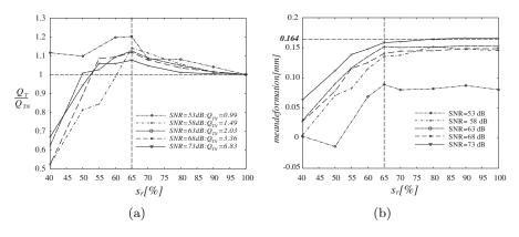
**Figure 5.** (a) Normalized  $Q_T (Q_{TN} = Q_T(s_r = 100\%))$  and (b) mean deformation of the test panel vs.  $s_r$ .
