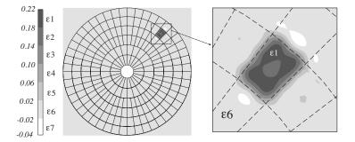
Figure 3. Gray scale map of the retrieved reflector surface for a distortion of 0.2 mm of the panel under test.
