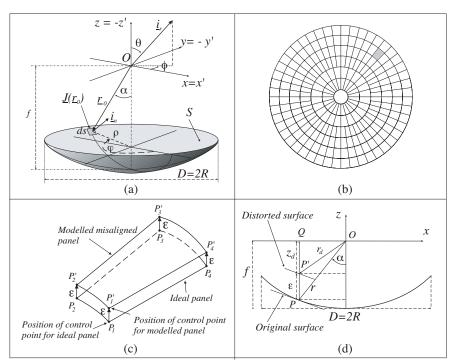
Figure 1. (a) Reflector Geometry; (b) front view of the parabolic reflector with subdivision into panels; the panel under test is highlighted in grey; (c) GRASP modelization of a panel; (d) description of the surface distortion.
