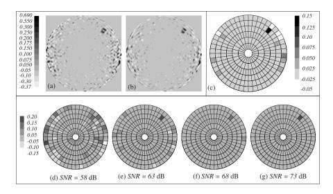
**Figure 4.** (a), (b), (c): gray scale map of the retrieved reflector surface for a distortion of 0.2 mm of the panel under test, SNR = 68 dB:(a) before noise filtering, (b) after noise filtering with, (c) all the distorted points of each panel in map (b) have been replaced by their mean value; (d), (e), (f), (g): gray scale maps of the retrieved reflector surface for a distortion of 0.2 mm of the panel under test for different values of the SNR.
