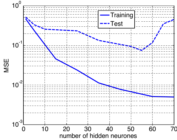
Figure 5. MSE obtained on training and test sets for different numbers of hidden neurones (imaginary permittivity) with MSE objective function.
