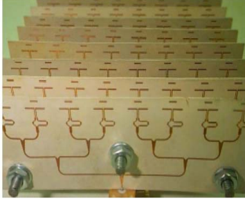
Figure 1. 2D quasi-Yagi antenna array with elements all pointing forward [3].
