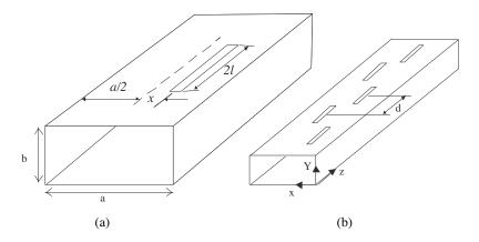
**Figure 1.** (a) A longitudinal slot module. (b) A linear array of N slots.
