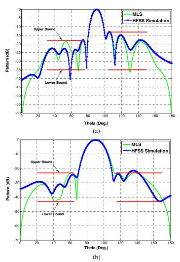
Figure 4. (a) 8 slots array with asymmetrical pattern, (b) 5 slots array with symmetrical pattern.
