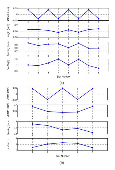
Figure 3. MLS Results for slots offset, length, spacing and excitation, (a) 8 slots array, (b) 5 slots array.
