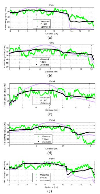
Figure 2. Comparison of the tuned model with the measurements and ITU-R P.1546 for measurement paths.
