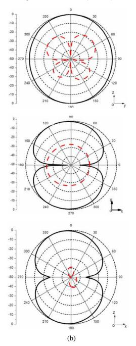
**Figure 6.** Radiation patterns of dual-band antenna with proposed CB-CPW at (a) 1.6 GHz and (b) 2.34 GHz.
