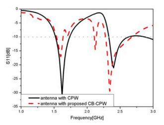
Figure 5. Return loss of dual-band antenna.
