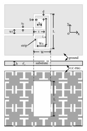
Figure 4. Geometry of dual-band antenna.
