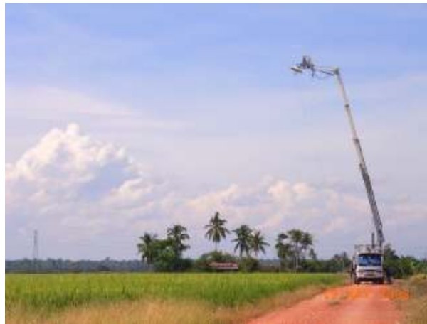
Figure 1. Ground-based C-band scatterometer during measurement trip.
