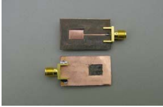
Figure 6. Photograph of the fabricated transition.
