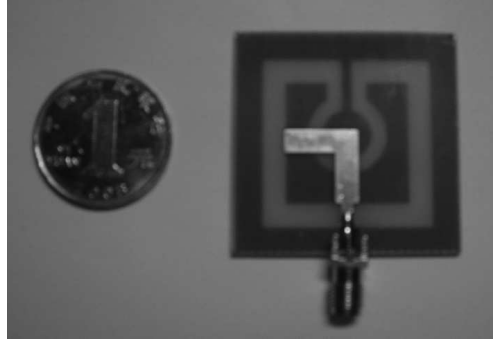
Figure 2. Physically realized module of the proposed dual-band slot antenna.
