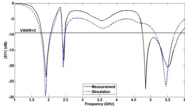
**Figure 3.** Return loss of the first antenna; measurement and simulation ( $\alpha = 143^\circ$ ).
