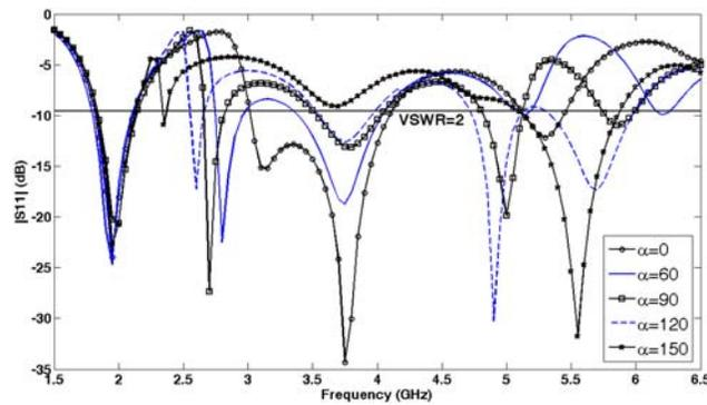
**Figure 2.** Return losses of the first antenna for five different opening angles ( $\alpha$ ) [deg].
