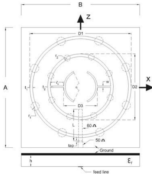
**Figure 1.** Geometry of the proposed triple-frequency annular-ring slot antenna.
