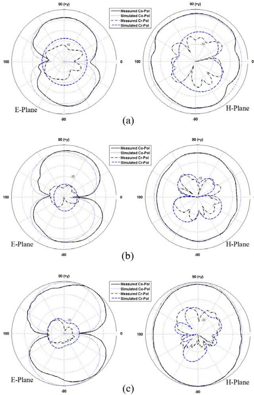
**Figure 5.** Measured and simulated  $E$  &  $H$ -plane radiation pattern of the first antenna (a) at 1.95 GHz, (b) at 2.44 GHz, (c) at 5.5 GHz.
