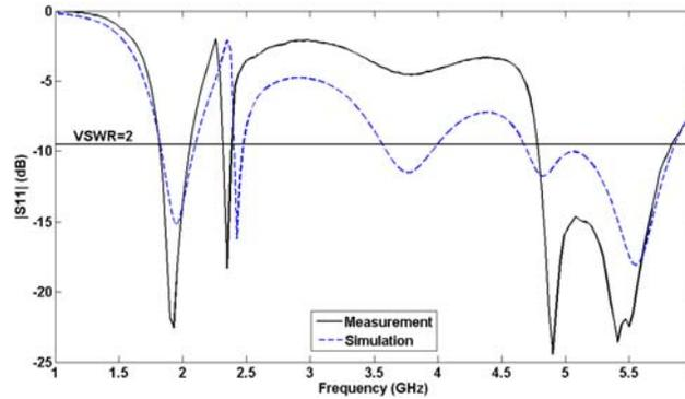
**Figure 4.** Return loss of the second antenna; measurement and simulation ( $\alpha = 145^\circ$ ).
