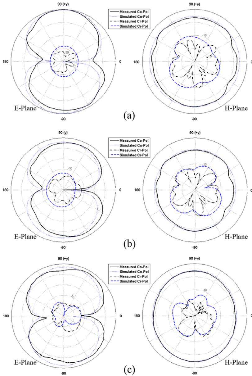
**Figure 6.** Measured and simulated  $E$  &  $H$ -plane radiation pattern of the second antenna (a) at 1.9 GHz, (b) at 2.44 GHz, (c) at 5.5 GHz.
