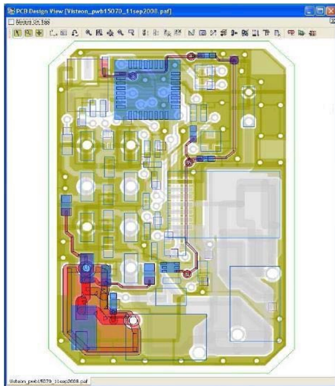
Figure 19. Extracted nets of the PCB: VCC, VPWR in red, GND in green.
