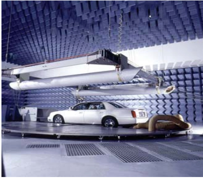
Figure 1. A photograph of vehicle level EMC testing.
