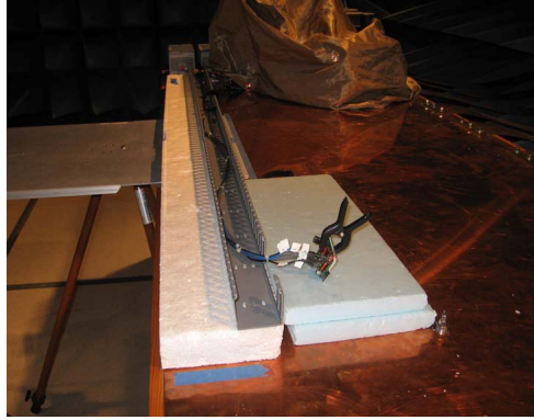
Figure 8. A photograph of the ECU, harness, and load inside the EMC chamber.
