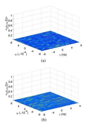
**Figure 9.** Cross-ambiguity function of the Colpitts oscillator with 3.5 GHz fundamental frequency, correlation interval  $T = 10 \,\mu s$ . (a) Cross-ambiguity function with different time. (b) Cross-ambiguity function with slight different parameters.
