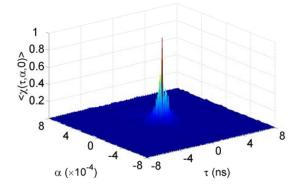
**Figure 6.** Auto-ambiguity function of the Colpitts oscillator with 3.5 GHz.
