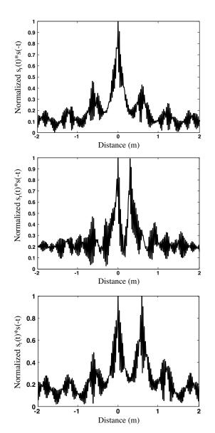
Figure 10. Calculated results of distance resolution of two objects using the experimental signal from the Colpitts oscillator with 1 GHz fundamental frequency. (a) Distance 0 m, (b) distance 0.3 m, (c) distance 0.6 m.
