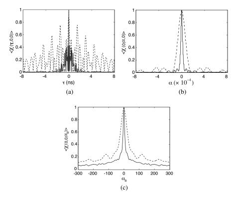
**Figure 7.** Slices of the auto-ambiguity function in Fig. 5 and Fig. 6. The solid line is the 3.5 GHz fundamental frequency signal, the dash line is the 1 GHz fundamental frequency signal. (a) Slices of  $\langle \chi(\tau, 0, 0) \rangle$ . (b) Slices of  $\langle \chi(0, \alpha, 0) \rangle$ . (c) Slices of  $\langle \chi(0, 0, \alpha_a) \rangle$ .
