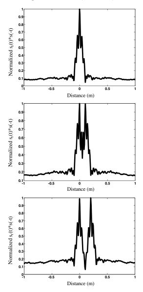
Figure 11. Calculated results of distance resolution of two objects using the experimental signal from the Colpitts oscillator with 4 GHz fundamental frequency. (a) Distance 0 m, (b) distance 0.1 m, (c) distance 0.2 m.
