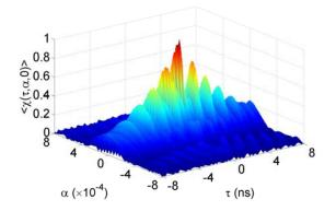
**Figure 5.** Auto-ambiguity function of the Colpitts oscillator with 1 GHz fundamental frequency.
