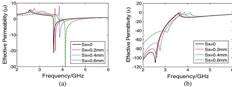
**Figure 4.** Real parts of retrieved effective permeability (a) and permittivity (b) under different relative slips  $S_x = 0, 0.2 \text{ mm}, 0.4 \text{ mm}$  and  $0.6 \text{ mm}$ .
