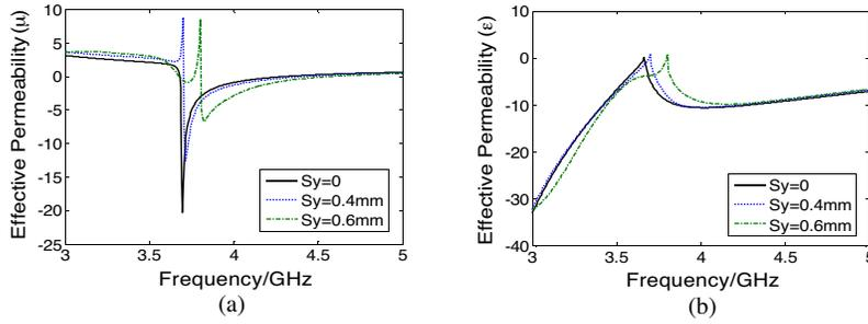
**Figure 5.** Real parts of retrieved effective permeability (a) and permittivity (b) under different relative slips  $S_y = 0$ , 0.4 mm and 0.6 mm.
