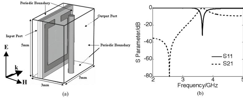
**Figure 2.** The MBC-SRR-based LHM unit cell without relative slips (a) and its transmission spectra (b).
