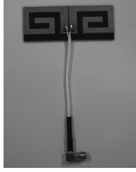
Figure 2. Photograph of a working sample fed by 50- \Omega coaxial cable.
