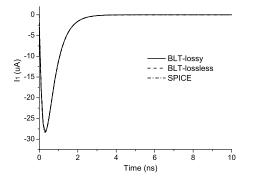
Figure 9. The transient current of the case in Fig. 7(b) with  $R_1 = 50 \Omega$  and  $R_2 = 100 \Omega$ .
