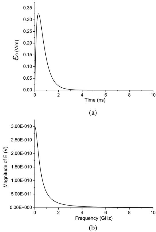
**Figure 3.** (a) The time waveform of the incident electric field; (b) The frequency spectrum of the incident electric field.
