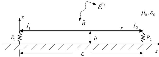
**Figure 1.** Single lossless line above an infinite, perfectly conducting ground.
