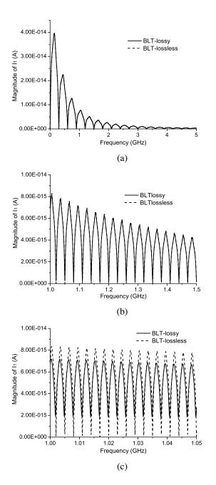
**Figure 4.** The frequency-domain current response of  $R_1$  with different lengths of the transmission line. (a)  $\mathcal{L} = 1 \text{ m}$ ; (b)  $\mathcal{L} = 10 \text{ m}$ ; (c)  $\mathcal{L} = 100 \text{ m}$ .
