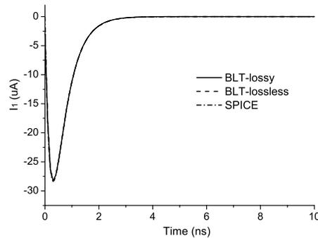
**Figure 9.** The transient current of the case in Fig. 7(b) with  $R_1 = 50 \Omega$  and  $R_2 = 100 \Omega$ .
