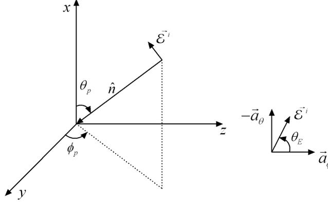
**Figure 2.** Definitions of the angles characterizing the incident plane-wave field.
