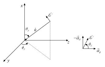
Figure 2. Definitions of the angles characterizing the incident planewave field.
