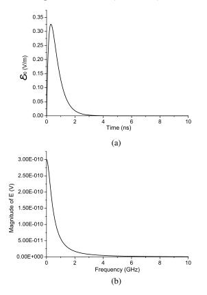
**Figure 3.** (a) The time waveform of the incident electric field; (b) The frequency spectrum of the incident electric field.
