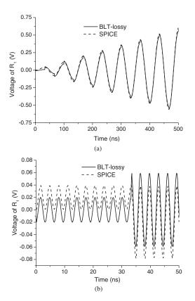
**Figure 11.** (a) The Voltage response of  $R_1$  when  $f_0$  equals 15 MHz; (b) The Voltage response of  $R_1$  when  $f_0$  equals 315 MHz.
