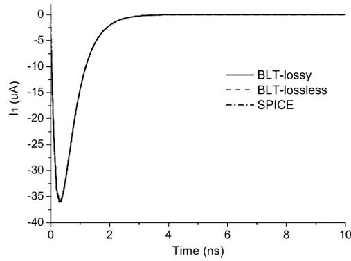
**Figure 10.** The transient current of the case in Fig. 6 with  $R_1 = 0 \Omega$  and  $R_2 = 0 \Omega$ .
