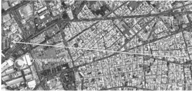
Figure 3. Experimental link between the School of Engineering, Aristotle University of Thessaloniki and the receiving site. The distance is about 2500 meters.
