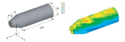
Figure 8. Induced normalised electric current on the surface of the Cone-Column, frequency 10 GHz, vertical polarization, at a incident angle of  $\theta_i = 60$ ,  $\varphi_i = 0$ .
