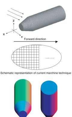
Figure 2. Schematic representation of graphical electromagnetic computing method in the illuminated and shadow region.
