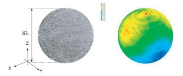
Figure 4. Induced normalised electric current on the surface of the sphere, frequency 10 GHz, vertical polarization, at a incident angle of  $\theta_i = 0, \varphi_i = 0$ .
