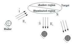
Figure 1. Geometry for bistatic scattering in the high-frequency region.
