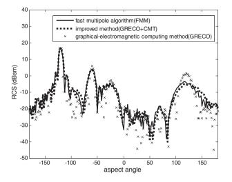
**Figure 9.** Bistatic RCS of Cone-Column, frequency 10 GHz, vertical polarization.
