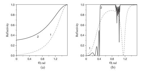
**Figure 6.** Reflectivity as the function of an angle of an incident wave.  $\omega = (a) 5 \cdot 10^{10} s^{-1}$ , (b)  $2 \cdot 10^{11} s^{-1}$ ,  $\varepsilon_a = \varepsilon_b = (1)1$ , (2)12.
