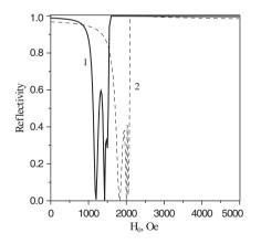
Figure 4. Reflectivity as a function of an external magnetic field (N = 20).
