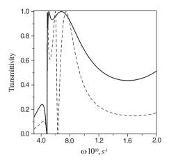
**Figure 10.** Transmissivity as a function of the frequency.  $\varepsilon_f = 5.5$ ,  $\omega_M = 3.11 \cdot 10^{10} \,\mathrm{s}^{-1}$ ,  $H_0 = 2000 \,\mathrm{Oe}$ ,  $\varepsilon_0 = 17.8$ ,  $\omega_p = 1 \cdot 10^{11} \,\mathrm{s}^{-1}$ , g = 2,  $d_1 = 0.002 \,\mathrm{cm}$ ,  $d_2 = 0.0005 \,\mathrm{cm}$ , N = 50.
