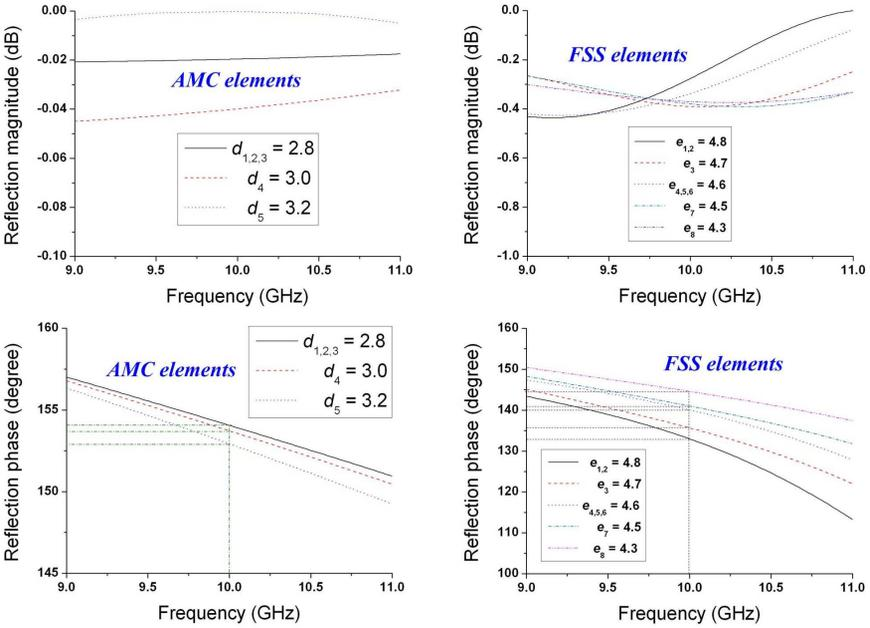
**Figure 3.** Frequency response of the reflection magnitude and phase on AMC and FSS.
