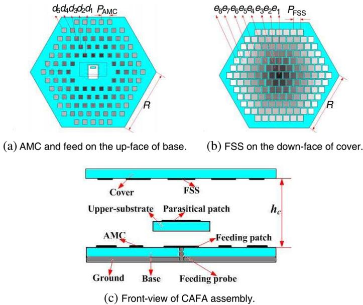
**Figure 2.** Structure of the printed CAFA antenna.
