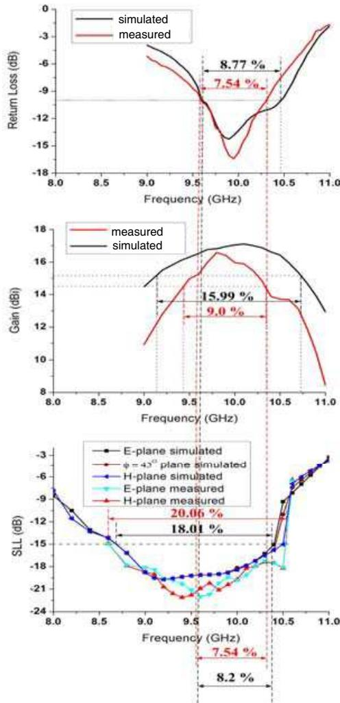
**Figure 4.** Frequency response of return loss, gain & SLL.
