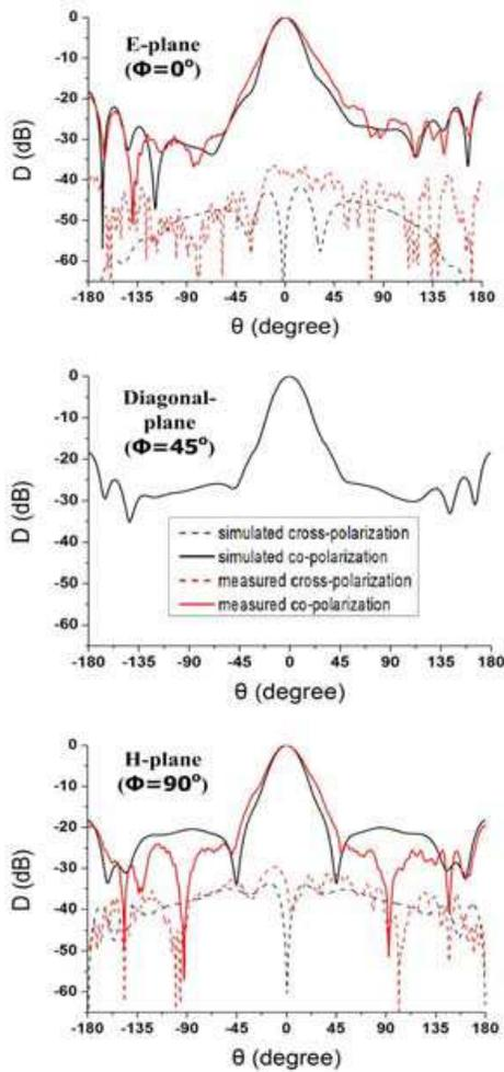
**Figure 5.** Radiation pattern of typical planes at 10 GHz.
