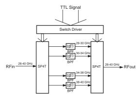
Figure 1. The block diagram of the ultra-wideband four-way switch filter module.
