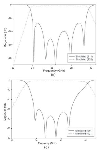
**Figure 4.** Simulated results of the designed three-line structure bandpass filters (a) filter one (26–30 GHz), (b) filter two (30–34 GHz), (c) filter three (34–38 GHz) and (d) filter four (38–40 GHz).
